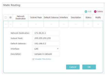
Network Destination: The destination IP address that you want to assign to a static route. This IP address cannot be on the same subnet with the WAN IP or LAN IP of Router A. In the example, the IP address of the company network is the destination IP address, so here enter 172.30.30.1.
